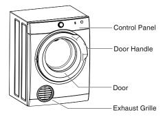
The exhaust grille has a range of positions, which allows you to select the optimum exhaust air angle. Simply hold the grille and rotate it until it hits the built-in stop.
